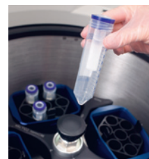
Fig 5. Spin adapters are used together with PD-10 Desalting Columns, PD MidiTrap G-25, and PD MiniTrap G-25 to enable use in a standard centrifuge.
