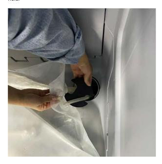
5 Press the bag flat on the bottom of the bin. Adjust the tubing from under the bin as needed and make sure the adapter and tubing remain in place.
