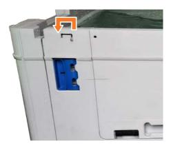
2 Push the drop-door upwards from the handles.
