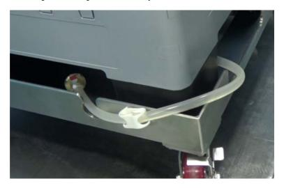
4 Fit the tubing adapter to the tubing and place the adapter on the discharge hole.
