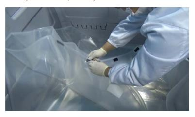
7 If you are using the 500 L/1000 L bin, close the drop-door and the latches before filling the bag.
