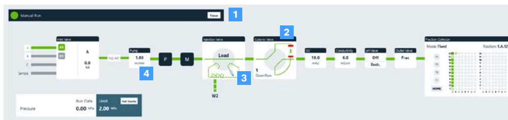
Fig 7. The Process picture represents the system flow path with a clear overview of placement of system components. All parts of the system are interactive and developed to ensure integrity of your run, samples, and columns.
