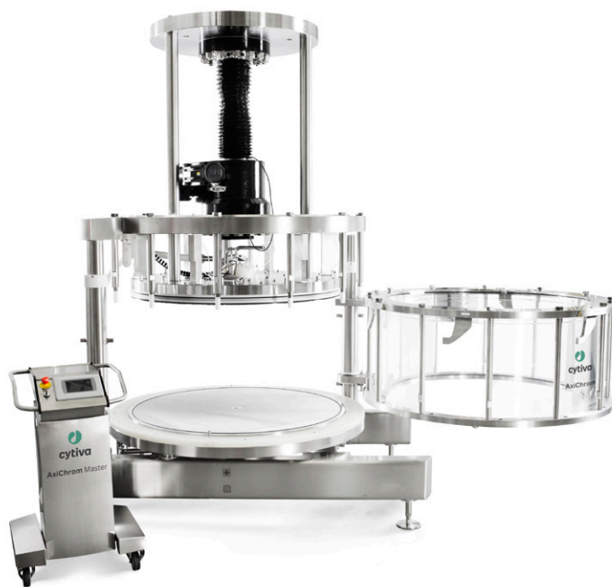
Fig 8. AxiChrom™ column in swing-out mode provides easy access to bed supports and O-rings. In multipurpose facilities, changing plastic bed supports for a new campaign is quick and hassle free.
