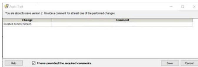
Fig 5. The audit trail is stored as an integral part of the file.
