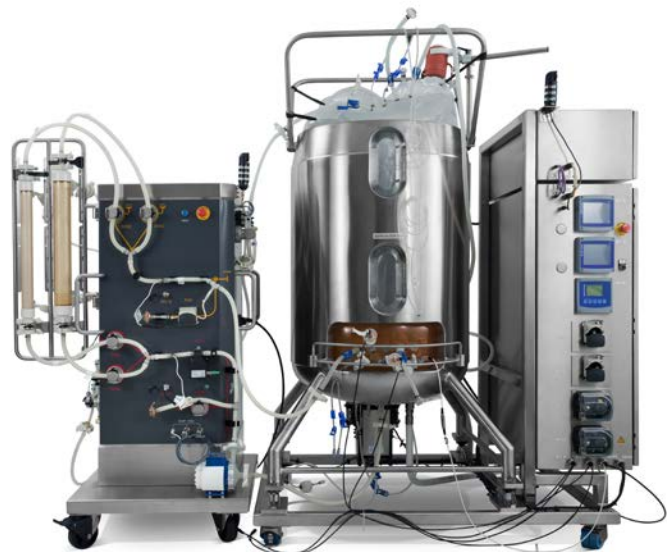
Fig 5. Xcellerex APS with Xcellerex XDR-500 bioreactor.
