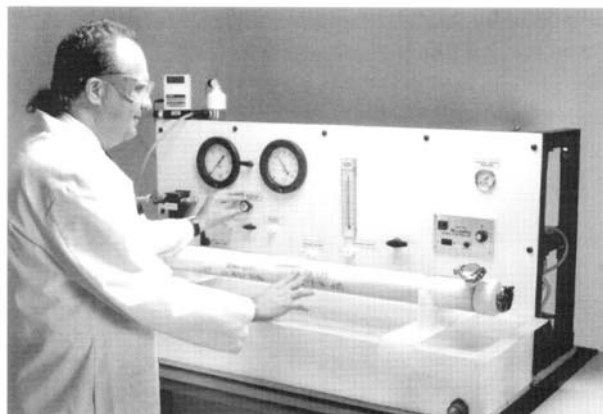
Stringent air diffusion specifications assure cartridge integrity.
